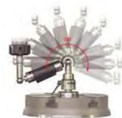
In practice, there are many factors in the machine geometry or the steering, which can cause effects on the radius of the test circle. More over, abrasion can lead to deviations from the circular shape.
