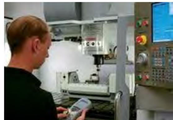
The QC20 creates a link between machine and diagnosis unit via Bluetooth which makes cables unnecessary.
